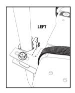
Install Side Pole Clamps loosely around Lower Strut tubes, and position inside Side Pole Clamp Bracket. Position 3 notches towards the main stilt body. Place the bolts in place (long bolt in back, and short bolt in front), and secure hand tight. Leaving this piece loose will allow you to slide the Upper Strut Tube over the Lower Strut tube in the next step. You will secure these bolts with the set of supplied wrenches in later steps.
