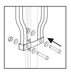
**Next**, secure each side with a 1½" bolt, two washers (one on the front and back of each bolt) and nylon locknut (HS124W).
