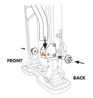
Insert Lower Strut Tube into the Outside Bracket on the main stilt body and secure with bolt, washers and nut. This view is from the rear of the stilt. The extra inside bracket is not used for single-sided stilts, but present in the event you want to upgrade and convert these stilts to double-sided stilts.
