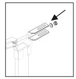
Remove nut and washer from bolt. Attach the second metal clamp bracket (HS131S) onto the main stilt body with the 3" bolt, washers and locknut (HS127W).
