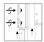
**Caution:** Do not pull the Inner Extension Tube past the "Max. Height" engraving, or force the Inner Extension Tube out of the Main Leg Strut. A plastic sleeve and tab is present to prevent this from happening, but excessive force will damage the plastic sleeve.
